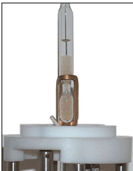
Fig. 1 High-pressure tube with Vycor porous glass and n-pentane in an NMR radio-frequency coil
